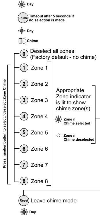
Chime is a low security monitoring system for use when the system is Unset. When a zone that is set to chime is operated, the internal sounder will produce a low volume two stage warning tone and the Zone indicator will show. The indicator may be cancelled by pressing Reset. Chime is particularly useful in a shop to warn of a customer presence or in a house to warn that a door or particular area has been accessed.
