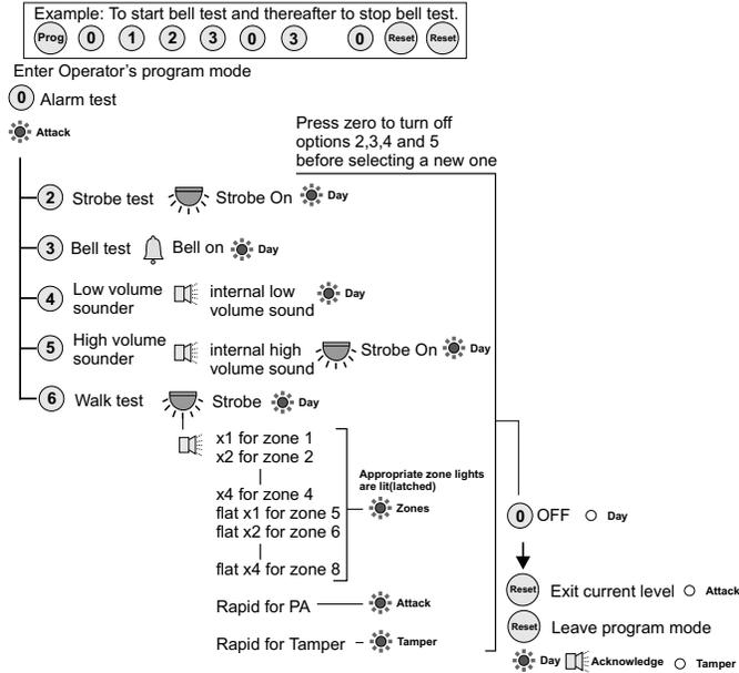
How to carry out Alarm and Walk tests
