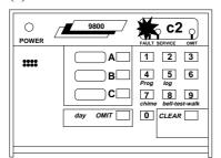
Go to a system keypad, then keyin your valid access code. The display will show the circuit which first caused the alarm, plus the 'Fault' and 'Service' lights. **(b)**
