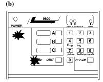
Press 'A'. Sounder emits a continuous tone. 'A' indicator flashes during exit time and remains on when set.
