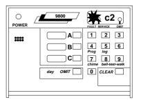
The display will have returned to the first circuit to alarm, e.g., 'c2'. Note: If you fail to write down the 'Control Code', repeat procedure (a) to (f)
