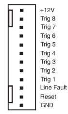
Figure 11. Trigger Header
