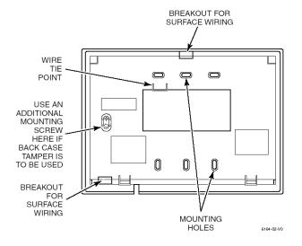
Figure 28. Wiring Entry (Back case)
