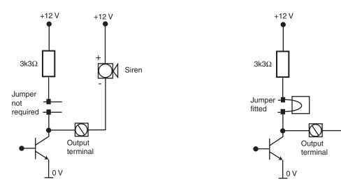
Figure 23. Output without jumper
