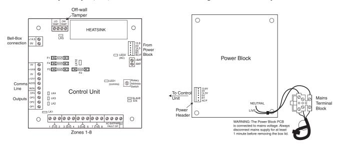
Figure 20. Power Supply Unit
