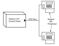
Figure 14. ECP Line - T Wire Configuration
