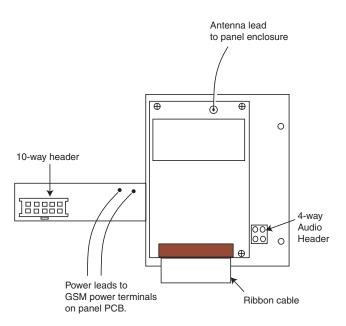
Figure 31. GSM Module - Top side
