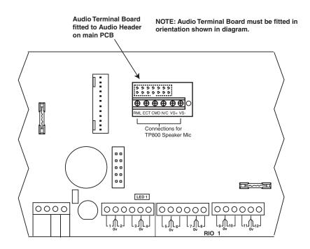
Figure 29. Audio Terminal Board fitted to PCB
