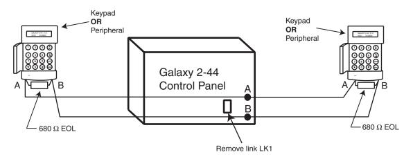
Figure 13. Twin AB Line Daisy-Chain Configuration
