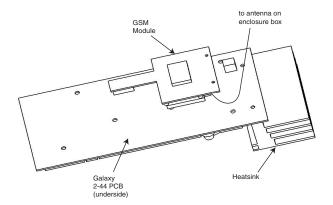
Figure 15. GSM Module fitted to underside of Galaxy 2-44 PCB
