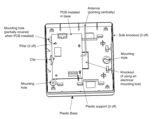
Figure 26. Plastic Base with PCB Installed
